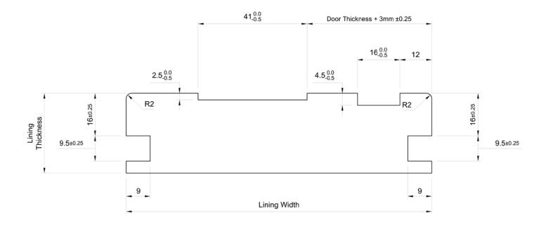
Do Not Scale. Description: MDF Lining - FD30 - 40mm Stop - Q2F To Both Faces - Acoustic
